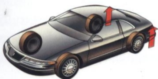
Air springs maintain the proper ride height and a smooth ride regardless of vehicle loading.
